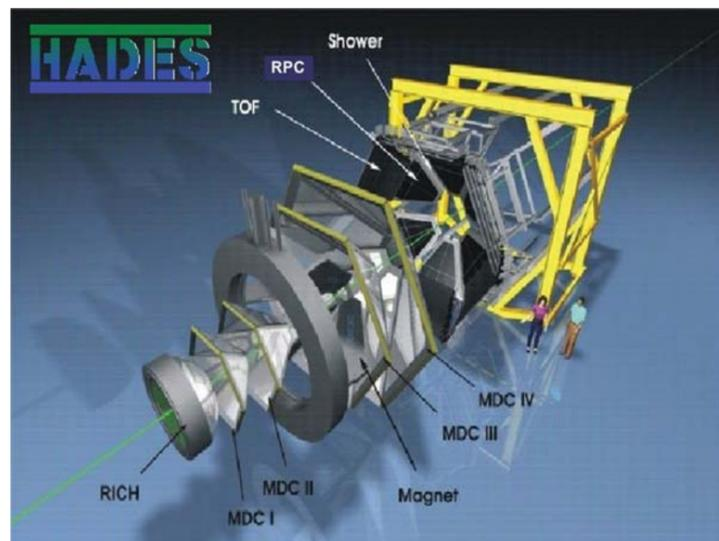
HADES is an installation of the first phase, which will work in experiments at the new accelerator complex FAIR, which will be built by 2018-19 year. The collabora-
