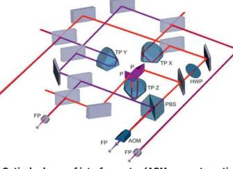
**Optical scheme of interferometer (AOM - acousto-optical** modulator, FP - collimating system, CR - triple prism, PBS – polarized beam splitter, P – prisms, I/2 - half-wave plate, M1,2,3 – mirrors for beam mixing). WORLD of MEPhI
