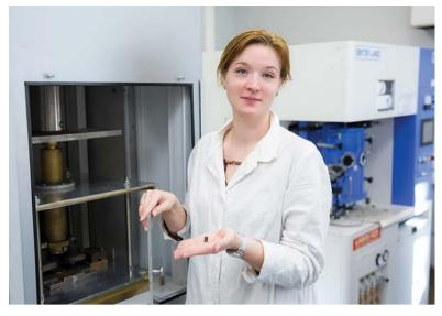
on electropower impact of powerful short-term (less than 1 msec) high-voltage electropulse and at the same time mechanical pressure on powder material. Material in the influence zone is warmed up to very high temperatures up to plasma condition. Pressure in the influence zone forms required properties of received products. The advantages of this technology are ecological cleanness, high efficiency: its energy consumption is 10 Electropulse method is based times lower than in the same
